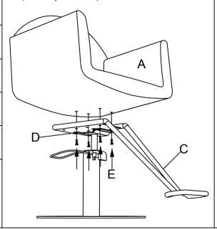
PartQty.DescriptionA1Chair topB1Base and hydraulicC1Footrest barD1BracketE5Bolt + washer + lock washer
